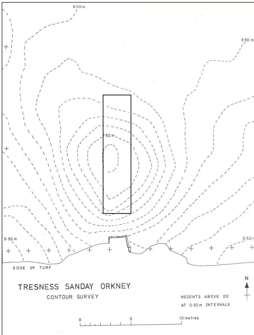
**Figure 2.** Contour survey of the monument at Tresness with the location of the trench (after Smith 1983)
