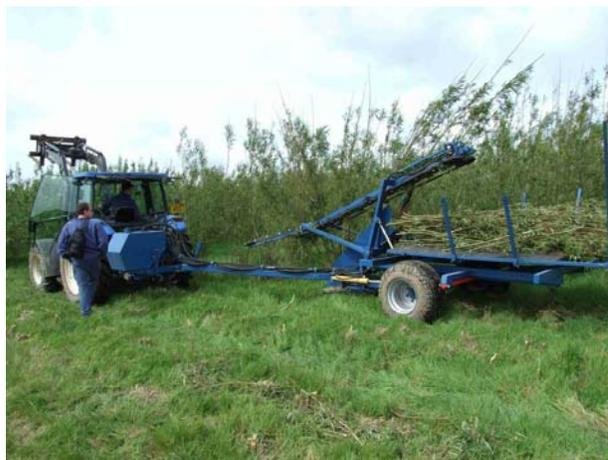
Prototype small-scale whole-rod willow harvester being tested on 3-year-old willow at Muddisdale.
