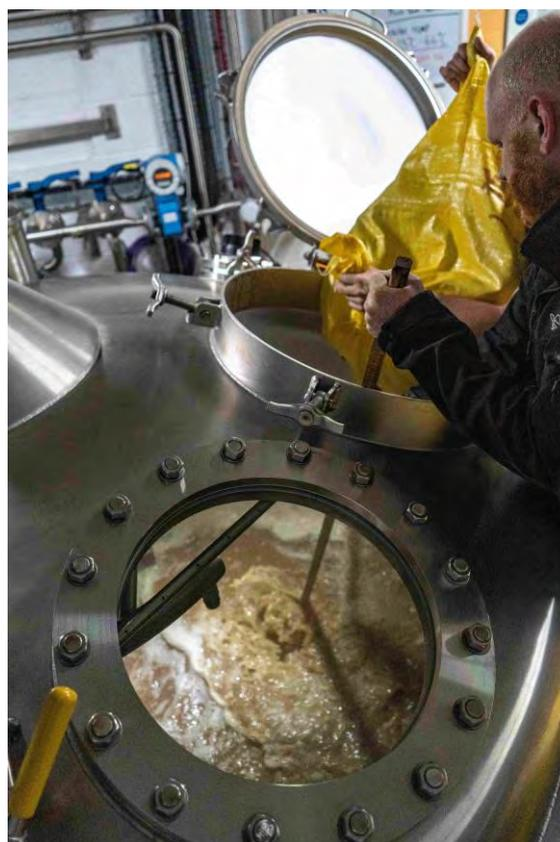
Malt made from barley harvested from the 2018 Raasay trial being added to the mash tun prior to distillation at Isle of Raasay Distillery in August 2019.
