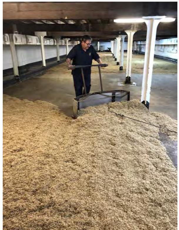
Barley from the 2019 Raasay trial being malted by Crisp Malt using their floor malting facilities in October 2020. The malt will be used for distillation by Isle of Raasay Distillery in 2021.
