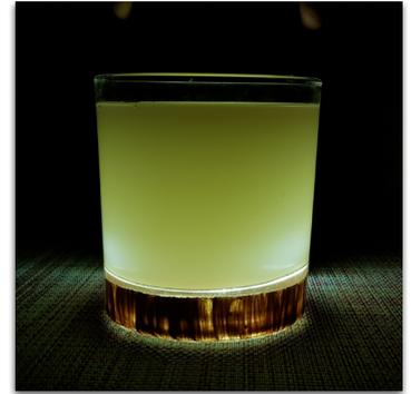
The milk is acting like the particles in the air and scattering the light so when you look at the torch light through the milk it looks red because the blue light has been scattered just like in a sunset!
